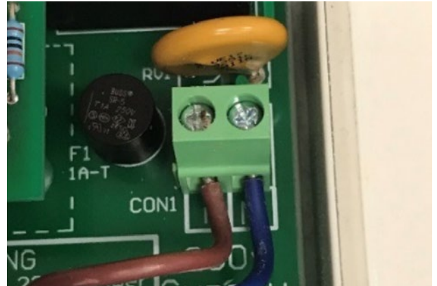
Figure 20: Prewired power cable on terminal block 1 (CON1).
